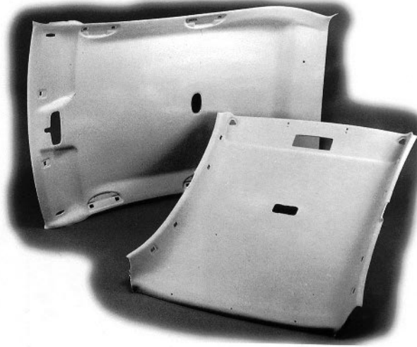
6.4 Automotive headliner covered with nonwoven fabric. Courtesy of Cosmopolitan Textile Company Ltd.
