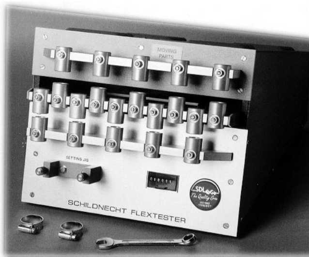
9.3 Schildnecht Flextester. Flexing is an important test for coated fabrics to assess polymer adhesion. Each fabric sample is clamped around two cylindrical holders, one above the gap and one below. The rails move rapidly up and down to flex the fabric sample. Reproduced with kind permission of SDL International Ltd.
