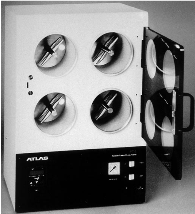
5.7 Atlas Random Tumble Pilling Tester. Photograph supplied by SDL International and reproduced with kind permission.
